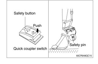
(3) Aligning the arm and bucket, insert static hook of quick coupler to the bucket pin.
