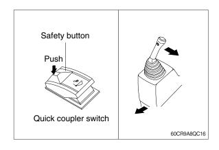
(6) After checking the connection status between bucket pins and hooks of quick coupler, insert safety pin of moving hook to lock position.
