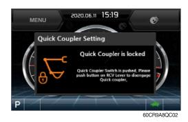
(5) To unlock the quick coupler, press the quick coupler button on the right RCV lever.
