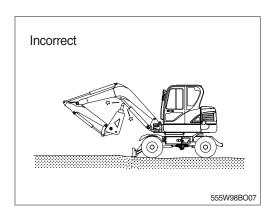
8) Do not extend the bucket cylinder fully and thrusting to raise the machine off the ground.
